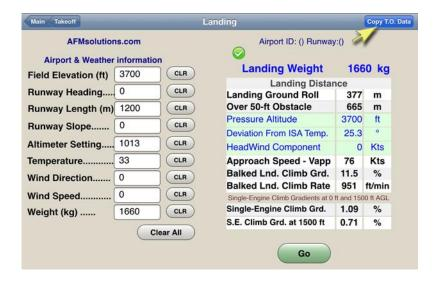
If the "Weight" box is left blank, the program will use the structural maximum landing weight allowed. If any of the Landing Distance results are out of range there will be a warning message shown in red. In the example above, the landing distance of 665 m is less than the runway length of 1200 m, so consequently we see a green checkmark next to the landing weight.
