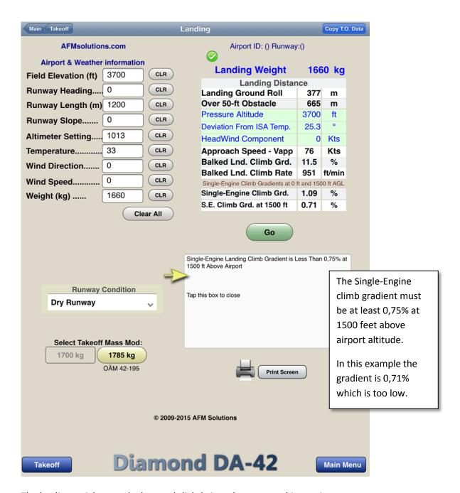
The landing weight must be lowered slightly in order to meet this requirement.
